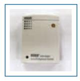
forts as low as possible. The data logger shown is from Onset but other manufacturers can provide similar loggers. This particular logger has one onboard temperature sensor, one onboard humidity sensor, one lighting level sensor, and two external jacks for other readings.
